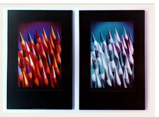
Both framed piece were exposed indoors for two years in direct sun daily for two hours. The left is framed with ACRYLITE® UV filtering sheet and the right is framed with glass.
