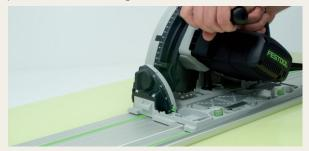
A guide rail or parallel stop is used to safely guide the circular handsaw.
