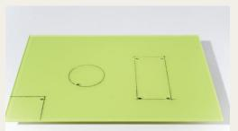
Always mark recesses and apertures on the masking film and predrill holes in the corners of cut edges.
