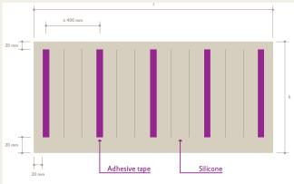
TIP: Pressing the sheet against the substrate using a level ensures that the silicone is evenly distributed and spreads to the thickness of the mirror tape. Care should be taken to prevent silicone from getting onto the adhesive tape.
