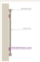
Principle: self-adhesive, flexible press-on fastener system.
